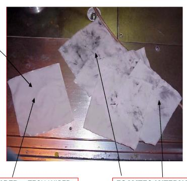
CURRENT FAB WIPER: TECH WIPED OUT SOURCE REGION UNTIL WIPER WAS NO LONGER REMOVING DEPOSITION FROM CHAMBER.
